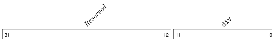
Figure 13.1: Format of sckdiv register.
