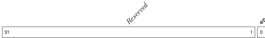
Figure 13.14: Format of fctrl register.
