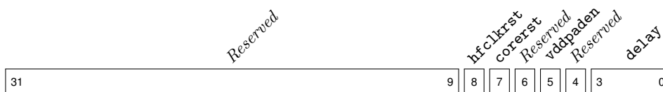
Figure 6.2: PMU instruction format.
